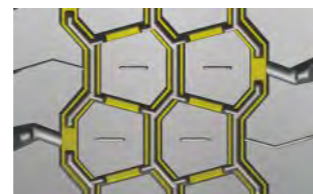
Circumferential tie bar design increase the stiffness on the shoulder area
